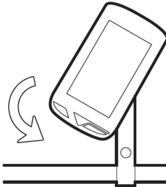
3. After securely locked, X5's camera will face front direction, same direction as the bike stem.
