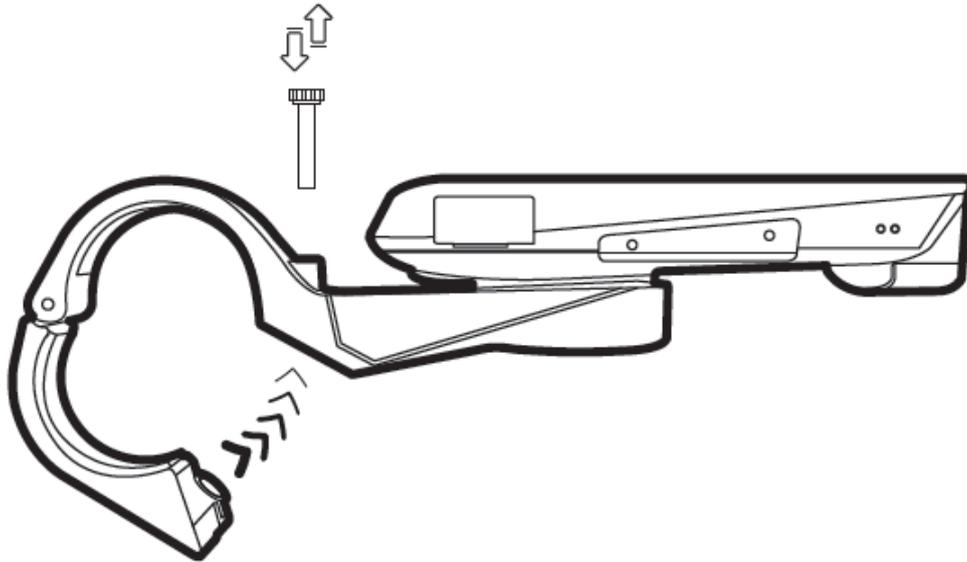
2. Place X5 toward right and align it with the bike mount; press downward and turn 90-degrees counterclockwise to lock it in the bike mount.
