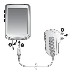
Figure 3. Connecting the charger to the Xplova G5
