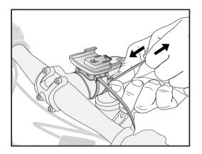
Figure 12. Attaching the mounting clip
