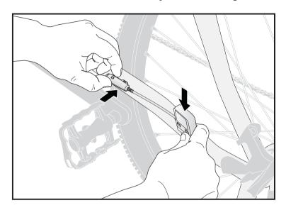
Figure 36. Positioning the combo cadence sensor
