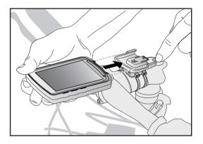
Figure 13. Attaching the Xplova G5 to the mounting clip
