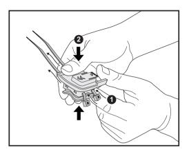
Figure 11. Threading cable ties
