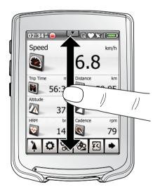
Figure 5. Switching views on the bike computer
