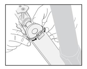
Figure 38. Attaching the cadence magnet to the left crank
