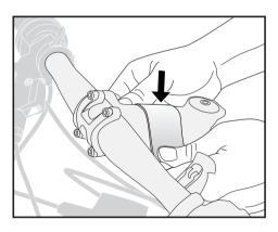
Figure 10. Applying the rubber sleeving
