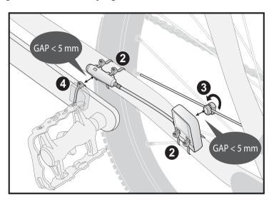
Figure 37. Attaching sensor and magnets
